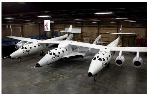
Fig. 1. SpaceShipTwo carried under White Knight Two
