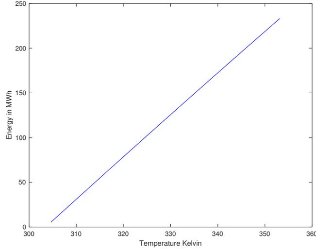
**Figure 9:** The energy needed to heat each layer of the storage to a temperature in accordance with the temperature profile, where the extreme temperatures are 80°C and 31.5°C.
