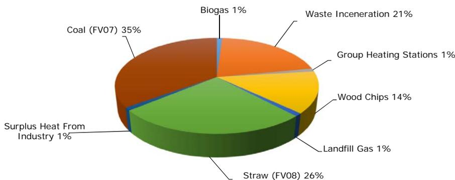
**Figure 1:** Illustration of the various district heating energy sources in *Fjernvarme Fyn*'s supply area in Odense and environs. [3]
