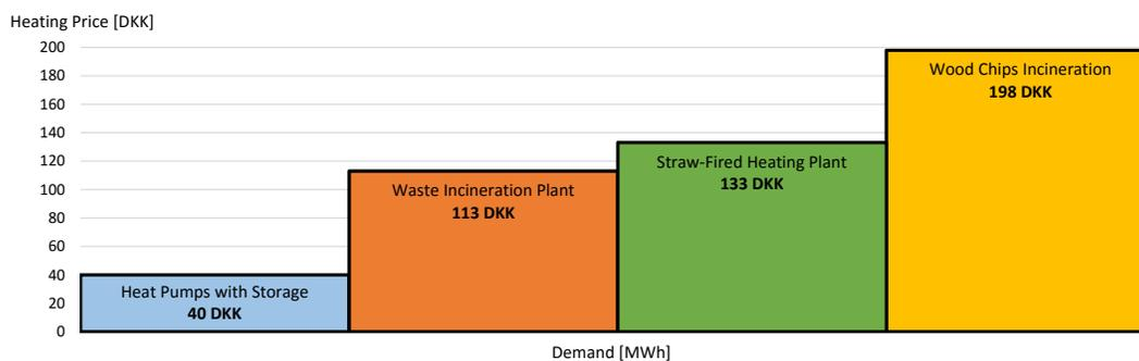
**Figure 13:** Illustration of the different sustainable production technologies in *Fjernvarme Fyn's* supply area and their respective prices. The supply amount is assumed to be the same for each technology.
