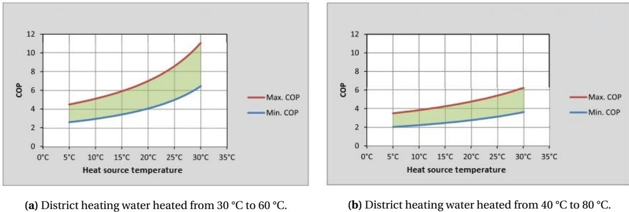
**Figure 6:** Expected COP for different district heating water temperatures. [14]
