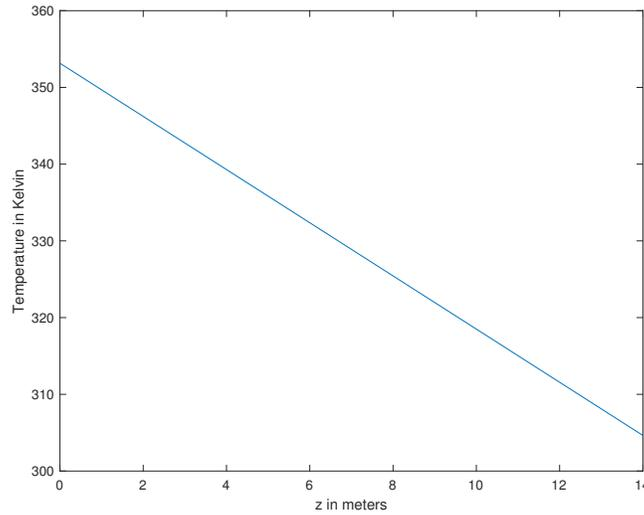
**Figure 8:** The temperature gradient depicted here is linear. The maximum and minimum temperatures of the gradient are 80°C and 31.5°C, respectively.
