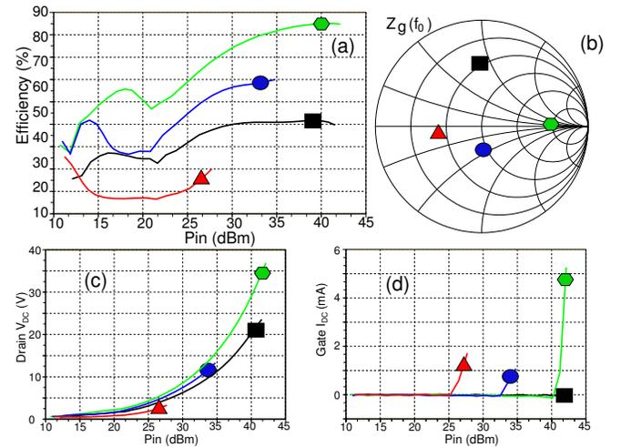
Fig. 12. Conversion efficiency, gate DC current and drain DC voltage versus input power for several RF load impedance values presented at the gate.  $V_{GS} = -4.4 \text{ V}$  and  $R_{DC} = 98.5 \Omega$ . The green point on the Smith chart corresponds to the highest efficiency point at  $Z_g(f_0) = (230 + j10) \Omega$ .
