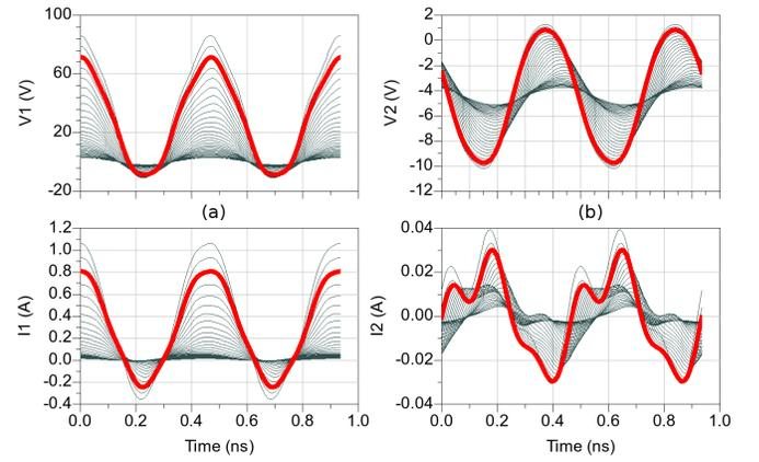
Fig. 11. Time-domain waveforms measured at drain (a) and gate (b) of the rectifier with  $V_{GS} = -4.4 \text{ V}$ ,  $R_{DC} = 98.5 \Omega$  and  $Z_g(f_0) = (230 + j10) \Omega$ . The RF input power at the drain is swept from 10 to 42 dBm, corresponding to the range of output power of the class-F<sup>-1</sup> PA.
