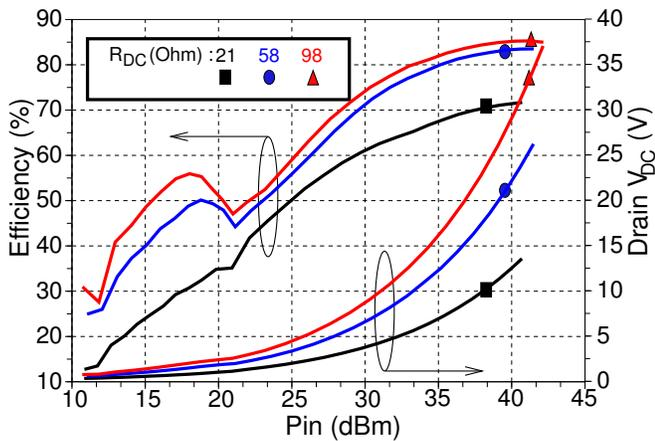
Fig. 13. Conversion efficiency and drain DC output voltage versus input power for several DC drain resistor values.  $V_{GS} = -4.4V$  and  $Z_g(f_0) = (230 + j10)\Omega$ . The highest efficiency of 85% is obtained at  $P_{in} = 40$  dBm with a  $V_{DC} = 30V$ .
