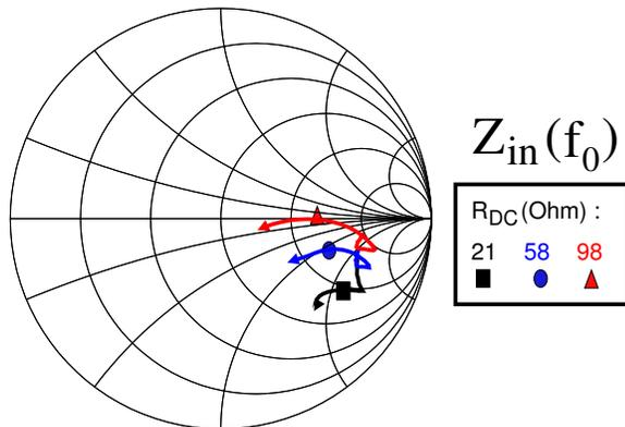
Fig. 14. RF impedance at  $f_0$  measured at the input (drain port) versus input power for several DC drain resistor values.  $V_{GS} = -4.4V$  and  $Z_g(f_0) = (230 + j10)\Omega$ .
