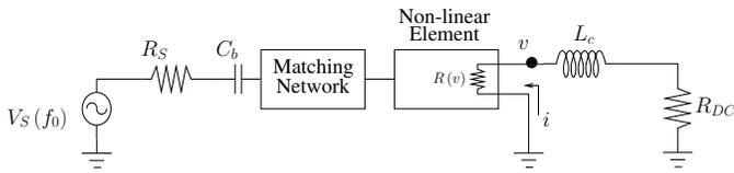
Fig. 1. Microwave rectifier circuit diagram. An ideal blocking capacitor  $C_b$  provides DC isolation between the microwave source and rectifying element. An ideal choke inductor  $L_c$  isolates the DC load  $R_{DC}$  from RF power.
